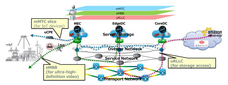
uRLLC: Ultra-Reliable and Low Latency Communications eMBB: enhanced Mobile Broadband mMTC: massive Machine Type Communication
